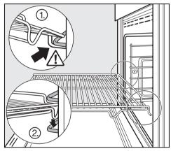
The racks are fitted with non-tip safety notches which prevent them being pulled right out when they only need to be partially pulled out.
